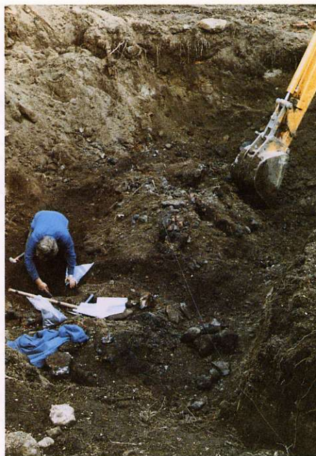
Back hoe trenching and sampling of the "C" vein mineralization
