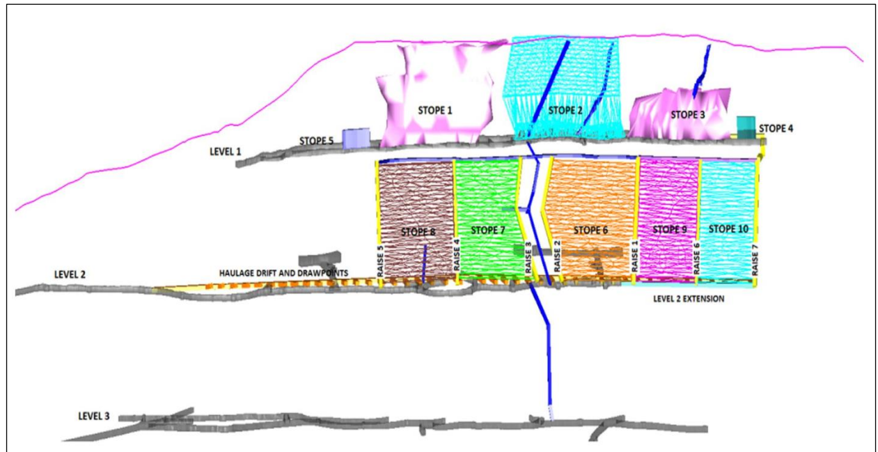
Figure 24: Cross Section of Underground Workings & Stopes at Treasure Mountain Mine (Source: Company Documents)
